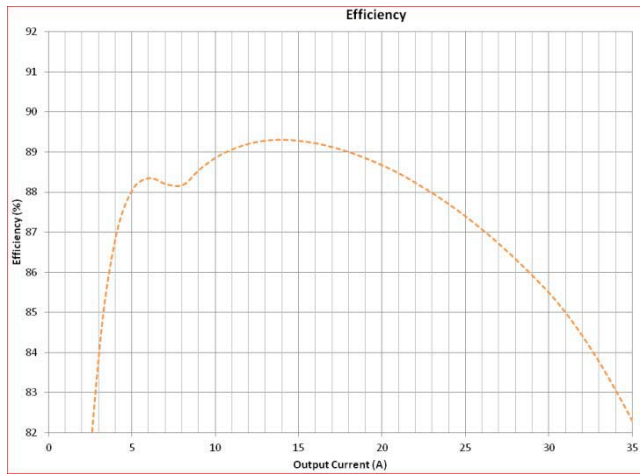
Figure 5. Efficiency – 19 V Input, 1.2 V Output, 500 kHz
